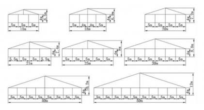
Main Frame: High reinforce aluminum, anti-rust surface, T6061/T6; It can be used for more than 30 years.
